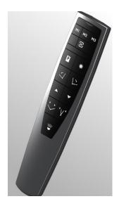
The keys M1 - M3 are memory keys and any position can be defined and then moved to automatically as with the iOS app. Move to the desired position and press the Memory button 3 times and then the desired memory position M1-M3.
